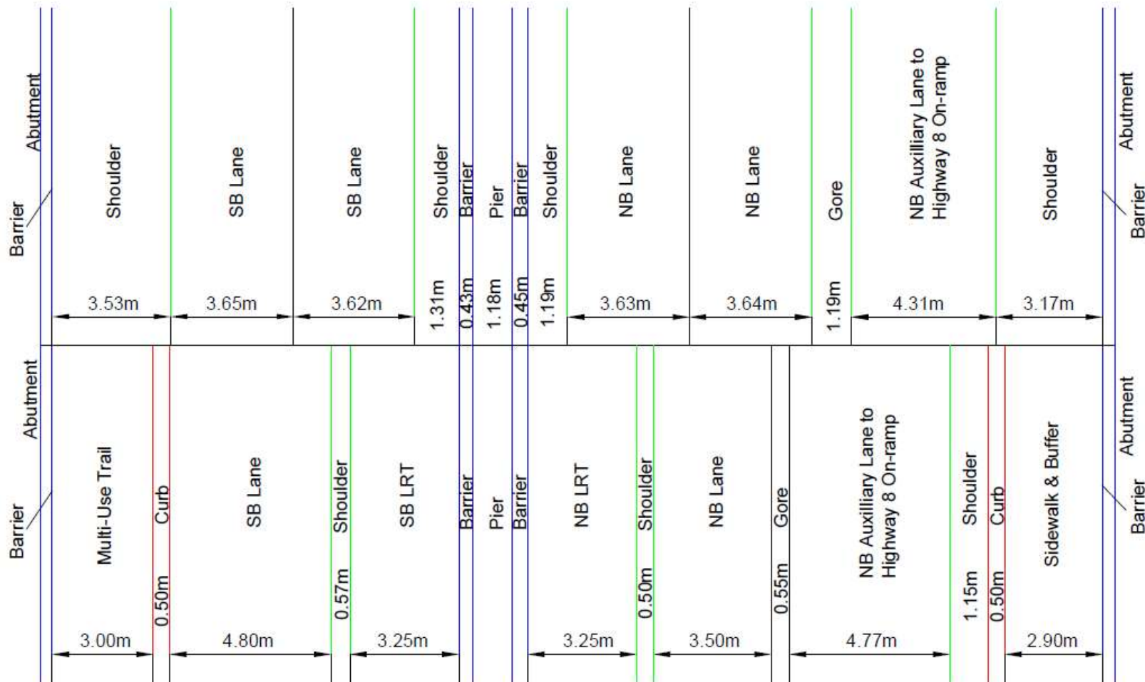
Proposed King Street lane configuration underneath Highway 8
